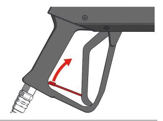
**3** Squeeze the handle to release the remaining pressure.
