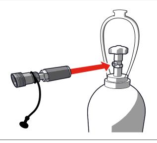
Connect the CO<sub>2</sub> hose to the CO<sub>2</sub> bottleto-hose connector on the CO<sub>2</sub> cylinder.
